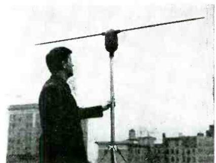
Figs. 4 (right) and 5 (left). Fig. 4 illustrates a 2-section dipole with a 1.8:1 tuning range, 46.5 to 85 mc. Length of antenna is 36" when closed, 66" when open. Fig. 5. Rotatable motor assembly of remote dipole. A, B and C represent control pin and gear mounts.
