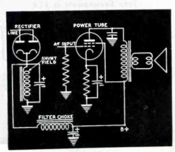
Fig. 5. A shunt-field filter circuit in an a-c/d-c receiver.
