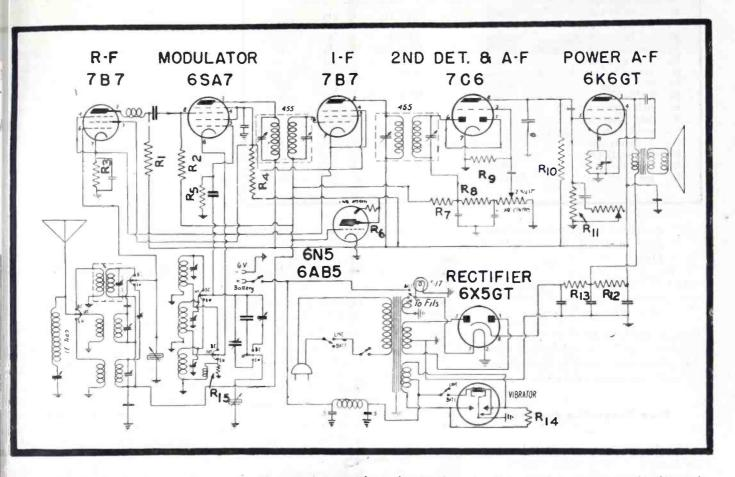
Fig. 1. A battery/a-c 7-tube super that employs fifteen fixed resistors for performing the various important functions described in this article.
