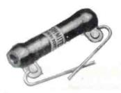
Fig. 3. A glass-insulated flexible resistor. Winding is on a fibre glass core encased in a braided fibre glass covering.
