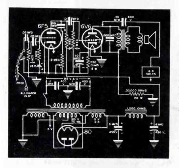
Fig. 2. An audio-frequency test amplifier. This unit can be used as an audio signal tracer. A shielded lead may be connected to the input. Audio voltages can be checked for intensity and distortion, and hum content or relative hum level.
