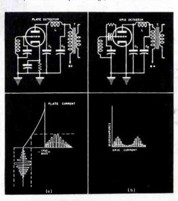
tection is illustrated here. In (a), since the tube is biased to cutoff, plate current will flow only on positive peaks of inbias the tube. This signal and the plate current is reduced
