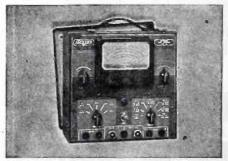
Electronic Multimeter—Model 645.
