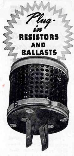
Troubled by fluctuating line voltage? Just plug in a Clarostat Automatic Line Voltage Regulator between set and outlet. At 110 volts the resistance of ballast is low. Voltage drop is negligible. But as line voltage increases, the resistance builds up so as to maintain a uniform and safe voltage delivered to the set.
