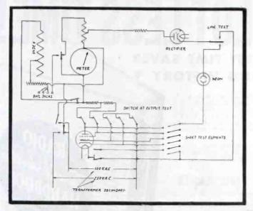
G.E. 2. The TC3 and 3P tube checker with individually operated lever switches to control voltage ranges from 1 to 117.
