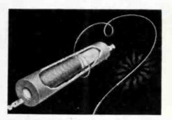
Fig. 5. Another recent form of resistor in which the wire itself is coated with a ceramic insulation before it is wound, the entire unit then being sealed in an outer-glazed ceramic shell.
