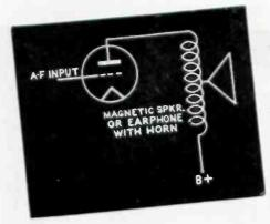
Figs. 1 (left) and 2 (right). In Fig. 1 we have a directly connected speaker in series with the plate supply. Fig. 2 shows an old type cone magnetic speaker in an impedance coupling circuit. The impedance coupling unit connected to the power tube eliminates d-c in the speaker.
