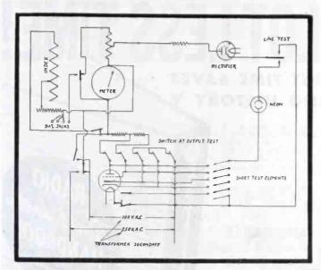
Fig. 2. The G.E. TC3 and 3P tube checker with individually operated lever switches to control voltage ranges from 1 to 117.
