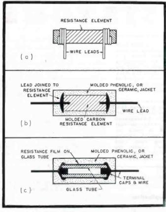
Fig. 2. Molded and sprayed-film type composition resistors. Above is a commercial type of non-insulated molded carbon resistor. (Courtesy Aerovox.) At left, (a), a crosssectional view of this resistor.
