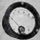
Weston 2 1/2" Model 506 Milliammeter D.C. 0-100
