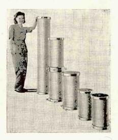
vegetable oil. The capacitors are b with adequately insulated and matched sections of uniform capacitance, connected in series. High-purity aluminum foil with a generous number of tab connectors is said to provide high conductivity with low inductive reactance. Capacitor sections are dried and impregnated under high vacuum in a closelycontrolled long cycle.
