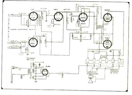
second audio contains the tone control circuits. The treble control uses a small and large coupling condenser, gradually cutting out the large one for an increase in treble. The bass boost introduces a regenerative feedback voltage from a divider on the output transformer through a low-pass filter to the 6N7G second audio grid. The filter consists of three elements
