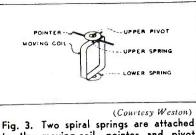
to the moving-coil, pointer and pivot assembly as shown in the diagram and illustration here.
