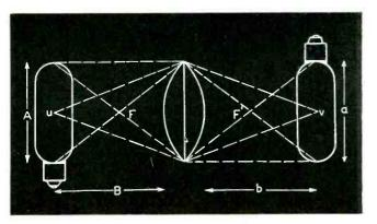
Fig. 3. How any lens can be constructed to possess two foci, F and F<sup>1</sup> at equal distances from the lens surface. F to center line is the focal length in one direction.
