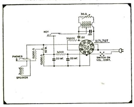
as an oscillation transformer, with a 30-ohm rheostat connected across the secondary for varying the frequency. The change in the resistance load is reflected into the primary, thereby varying the inductance. A .03-mfd tuning condenser is permanently connected across the primary. The key is located in the B+ circuit, so key and ground must not be touched at the same time.
