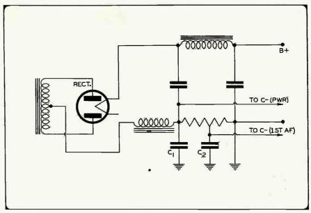
Fig. 7. Large receiver bias bypass system.
