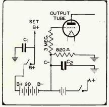
Fig. 6 (top). Battery bypasses. Fig. 8 (bottom). Battery a-c/d-c fil. circuit and a-f bypasses.
