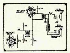
Fig. 4. RCA Victor 55X with e-m and p-m speaker units.
