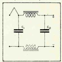
being for high voltage (600-volt peak). They are wound similar to a paper condenser, in rolls. Any waterproof container may be used; hence, we see metal being replaced with cardboard and plastics. In wets, the metal container acted as the cathode as well as container for the electrolyte but, when used with drys, it had no active purpose. When properly formed, drys have an insulation resistance of many thousand megohms per square centimeter area.
