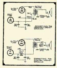
Fig. 3. Circuit changes in RCA Victor IX, 12X and 14X for p-m replacement.
