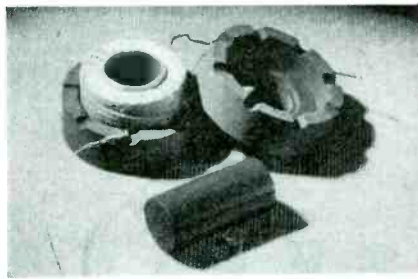
Crolite powdered iron core and shield, with coil inserted. The core at front slips into center of coil and shield. Slots in the shields accommodate the coil connections.
