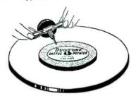
needle sharpener which utilizes the turntable of the phonograph motor for drive power.
