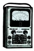
age ranges, at 1,000 ohms per volt; 4 current ranges, 3 resistance ranges to 5 megs and 6 decibel ranges. All connections lead from only two pin jacks, with the exception of the 1,200 and 6,000 volt ranges. A 400 microampere rectangular indicating meter, and wire-wound multipliers are em
