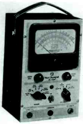
Fig. 3. The VoltOhmyst is an electronic voltohmmeter that has provisions for a-c measurements and other multimeter functions.
