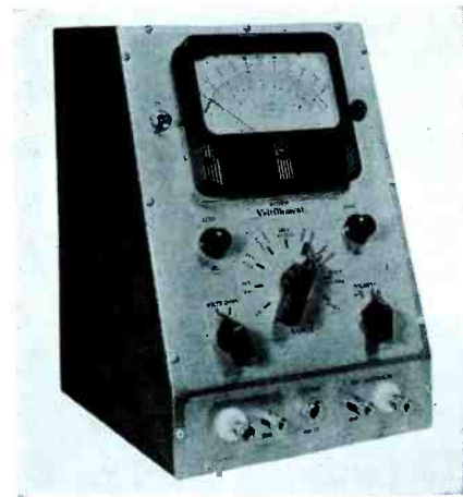
Fig. 2. A single adjustment of the ohmmeter zero point is all that is required for every range of the instrument.
