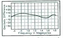
Fig. 2. A properly installed antenna of the noise reducing type will deliver an average net gain in input signal level over an antenna of the same dimensions without noise reducing transformers.
