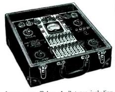
future types. Tubes of all types including gas rectifiers may be tested as well as pilot lamps and Christmas tree lights. Three ranges are also provided for testing bat-Three teries and d-c power supplies. The instrument is available in counter or portable models. Additional information and prices may be obtained directly from Radiotech-nic Laboratory, 1328 Sherman Ave., Evanston. Ill.
