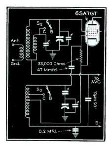
Fig. 2. In the G. E. HJ612 the antenna input transformer is shifted by paralleling the two secondary windings while part of the oscillator inductance is shorted.
