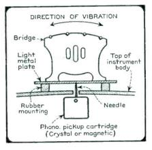
Fig. 4. Vibration pickup.
