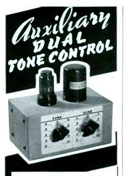
A simple circuit gives you an effective tone compensating system to boost or attenuate the bass and treble frequencies independently of each other. It may be incorporated in your present amplifier or receiver.
