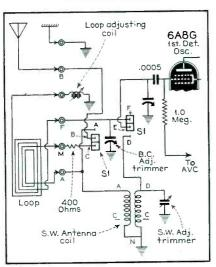
wave tickler having in series a 35-mmfd by-pass condenser. On the broadcast band, the shunting effect of the short-
