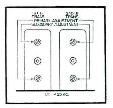
i-m receivers. The limitations of ordinary test equipment, possessed by even the more advanced Service Men are such that alignment in the field should not be attempted unless it is absolutely necessary. If alignment is attempted, the manufacturer's instructions should be followed to the letter.
