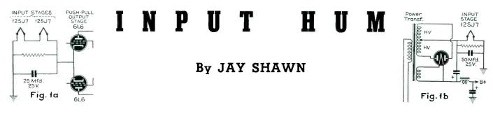
O NE of the more frequent difficulties encountered in high-gain public address amplifiers is input hum. In servicing amplifiers of this type much time can be wasted only to find that the trouble appears to be centered in the input stage. Shorting the input grid to ground does not clear up this condition, in some cases the hum actually becomes worse... This indicates trouble after the grid, but when the plate supply is opened up the hum stops.
