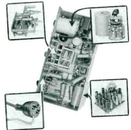
Output available at end of coaxial cable speeds work, eliminates long extension cords in single stage work or i-f gain measurement, minimizes leakage. Fully shielded, these 10 band magnetite-core coils and airtrimmer capacitors make possible excellent accuracy and stability of dial scale calibration.
