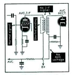
Fig. 5. A check of a receiver with a defective avc circuit quickly discloses the fault as being due to a shorted primary winding in the avc i-f stage. The signal tracing instrument showed normal signal at the grid of the avc i-f tube but no signal at the plate, thereby isolating the trouble.
