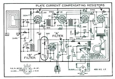
Fig. 3. The Crosley 549 uses a miniature lamp as an A filter (above).
