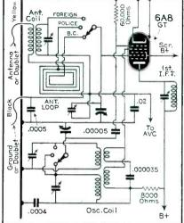
Fig. 4. Crosley 729 makes use of the image frequency to cover the police band. Note that the oscillator coil remains unchanged for this band.
