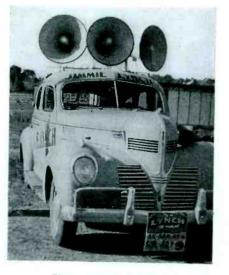
Photo courtesy University Laboratories. Fig. 3. (Above.) Jimmy Lynch uses a 60-watt mobile sound system with three horns to ballyhoo for his Death Dodgers at the New York World's Fair.
