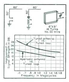
Fig. I. Both the tuned and the untuned types of outdoor antennae will definitely deliver considerably more signal to the input posts of a radio receiver.
