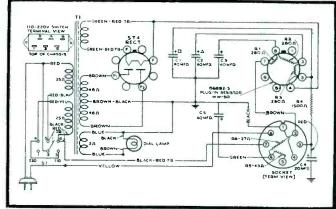
Fig. 10. RCA 4QB, 4QB4, four-tube, lowdrain farm sets employ a 1A7G for short wave reception; the former model for two such bands.
