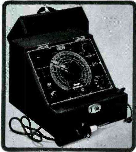
Fig. 3. The hinged cover of the Exam-eter is removable and reveals the sloping panel and the direct reading scales.
