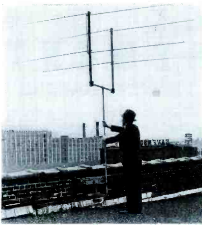
Fig. 19. A four-pole television antenna array, such as the RCA type shown, is used in localities with very high noise level and low signal strength.
