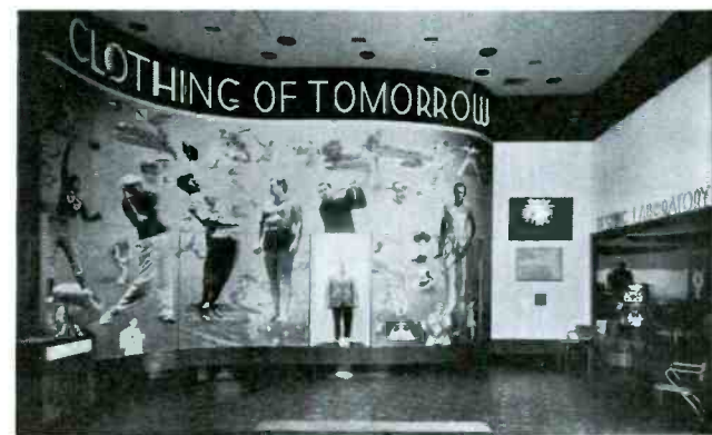
Fig. 16. Clothing dummy robots are made to talk and move, the movements of their lips and other parts perfectly synchronized with the speech by Robophone, a combination sound system and mechanical control device in which synchronism is insured by sound discs which carry both speech and controlling impulses.
