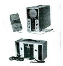
The alignment oscillator is a newly developed instrument for visual alignment of the r-f and i-f circuits in television re-ceivers. The calibrator and the oscillograph have many applications for other high frequency work, it is said. Additional information may be obtained directly from RCA.
