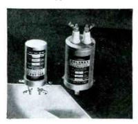
capacitor for general amateur transmitter use. This unit, available in standard values, is built of paper sections which are oil-impregnated under high-vacuum. They are assembled in insulated round metal cans, oil-filled and hermetically sealed. Terminals are procelain stand-off insulators. Mounting is accomplished by means of detachable rings.
