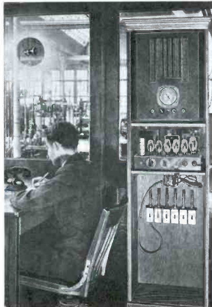
The reader in an American plant is a Lafayette radio and 30-watt amplifier with the output distributed through six speakers.
