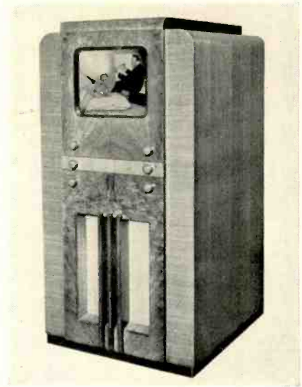
The DuMont 180 series of television receivers employ 22 tubes including a 14-inch electro-statically deflected cathode-ray tube.
