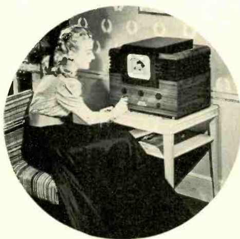
RCA TT5 reproduces television images and utilizes the chassis and speaker of any a-c receiver for sound. A 5-in c-r tube is used and 16 others.
