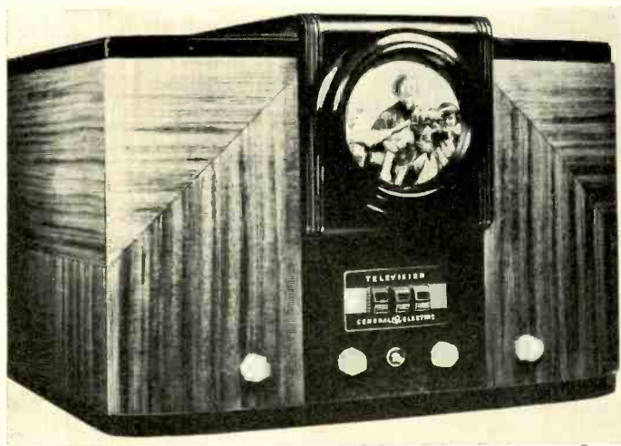
G.E. Model HM171 (above) table model has a 5-inch picture tube, is used for sight and also as a sound converter. It employs 17 tubes and covers three television bands.
