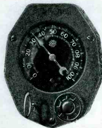
Fig. 4. Early type remote control heads mounted on the steering column.
