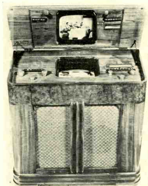
The Stewart-Warner console (below) combines all-wave sound with a television receiver. It employs a 12-inch picture tube.
