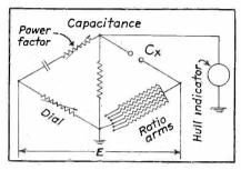
Fig. 5. Condenser analyzer part of bridge circuit.
