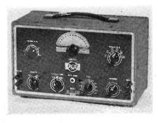
Fig. 4. The RCA model 150 test oscillator in its portable carrying case. Front view showing dial and panel arrangement.
