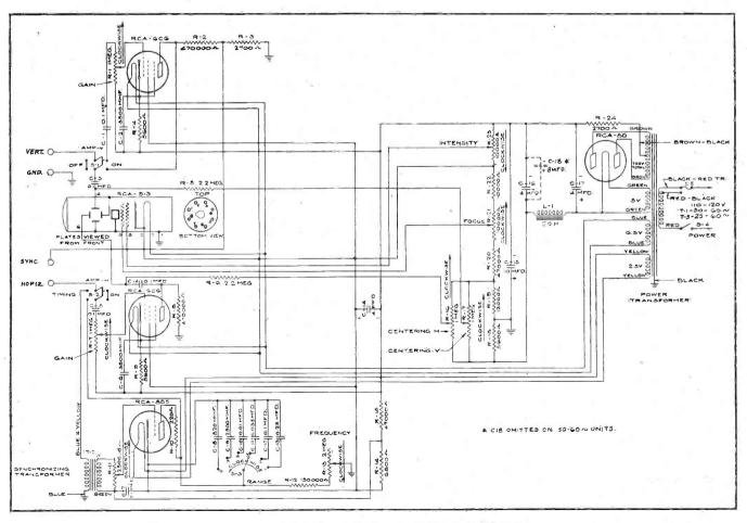
Fig. 3. The RCA model 151 carhode-ray oscillograph circuit diagram.
