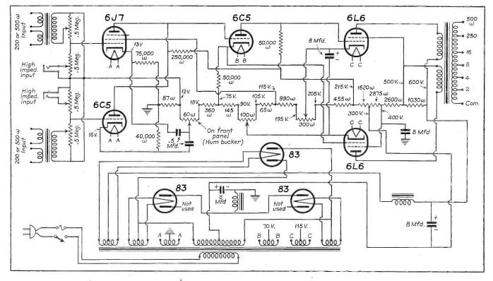
Fig. 6. The complete beam-power amplifier.
