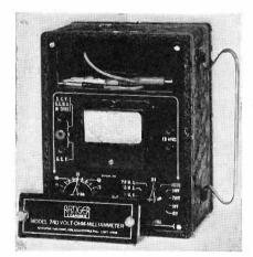
volt; (d-c accuracy 2 per cent, a-c, 5 per cent) 1-10-50-250 d-c milliamperes; 0-300 low ohms; high ohms to 250,000 at  $1\frac{1}{2}$ volts. Provision for higher resistance readings by addition of external batteries.
