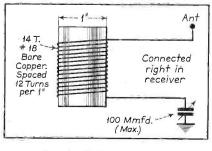
Fig. L. Series wave trap.
