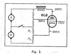
is not to be confused with a phase inverter) which is capable of driving two 6L6 tubes in true push-pull fashion.
