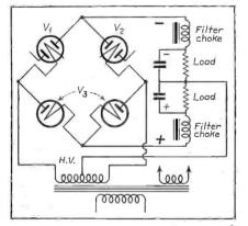
Fig. 1. Stabilized bridge type rectifier system.
