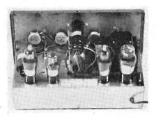
Fig. 2. The rear of the RCA model 151 cathode-ray oscillograph with the case removed, showing positions of parts and tubes.
