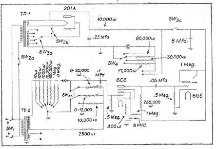
Fig. 4. Tobe a-c bridge-analyzer circuit.
