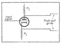
Fig. 4. Direct-coupled signal divider circuit.
