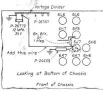
This modification was put in effect at the factory in all 160-P and 180-L receivers, and in all 160-L produced after October 23, 1936,
