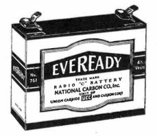
This is a No. 761–4<sup>1/2</sup>-volt General Purpose Battery. The size and composition of the cells in this battery make it suitable for such purposes as filament current supply for two 2-volt tubes in series, microphone battery, relay battery, and other uses where the No. 771–4<sup>1/2</sup>-volt Radio "C" Battery is not recommended.
