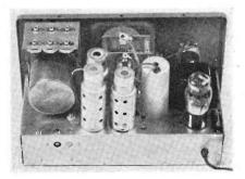
Fig. 5. The rear of the RCA model 150 test oscillator, showing positions of parts and tubes.
