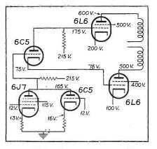
Fig. 5. Voltage distribution in the amplifier.
