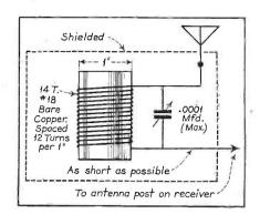
Fig. 2. Shunt wave trap. \*
