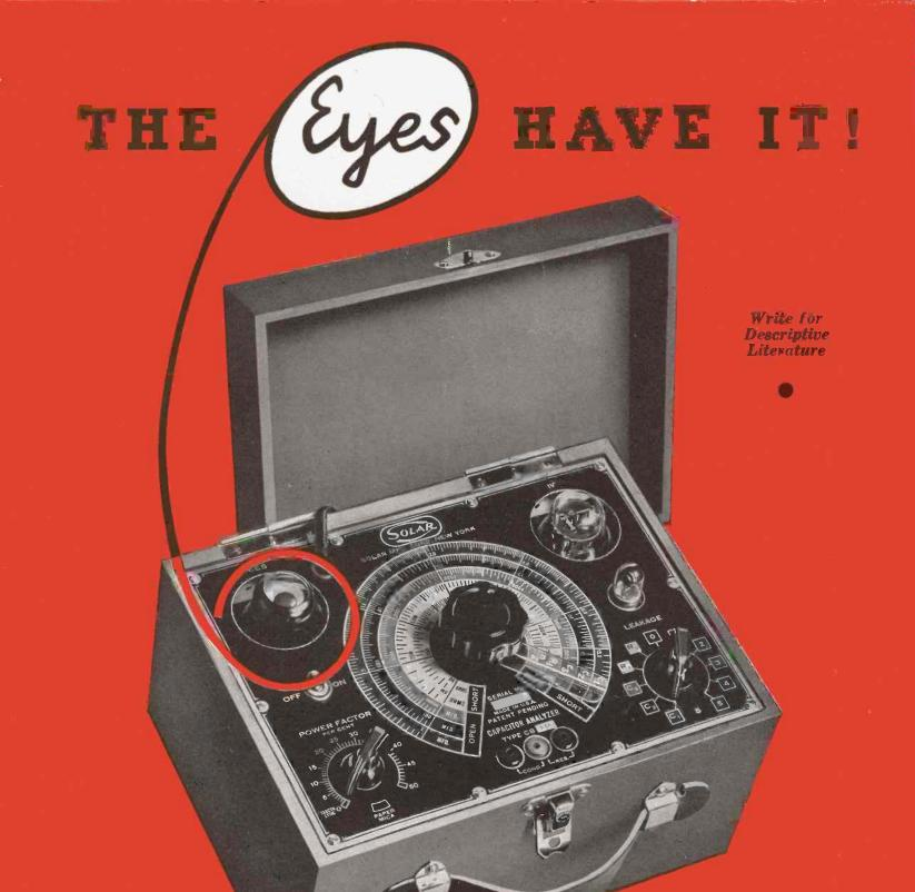
Your eyes and the MACIC TUBE .... see all, know all, quick as a wink! Capacity, power factor, leakage, resistance, read directly on the panel. SOLAR CAPACITOR ANALYZER
