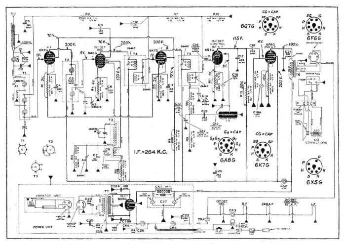
Fig. 1. Atwater Kent 556 circuit diagram.
