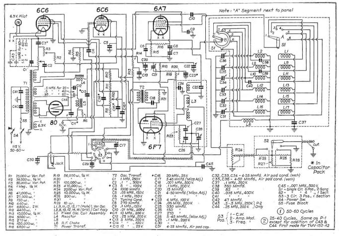
Fig. 6. The RCA model 150 test oscillator circuit diagram.
