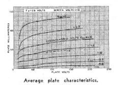
design of the 25L6. The design is similar to that of the RCA-6L6 with the difference that the 25L6 is intended especially for operation in a-c, d-c receivers.
