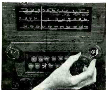
Fig. 1. A small set-up knob is located behind the tuning selector knob.
