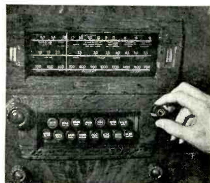
Fig. 2. Rocking the set-up knob while pulling it out will mesh the gears.
