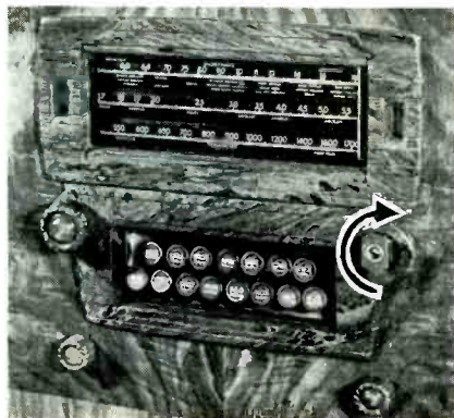
Fig. 3. A definite stop is reached at the extreme end of the clockwise rotation of the set-up knob.
