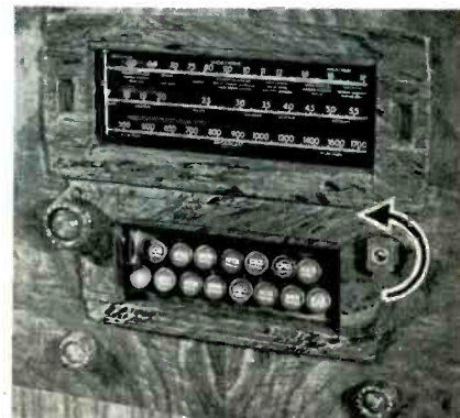
Fig. 6. A definite stop is reached at the extreme end of the counter-clockwise rotation of the set-up knob.
