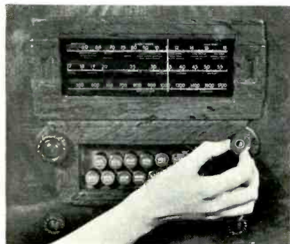
Fig. 5. The stations are preset by tuning them with the set-up knob.
