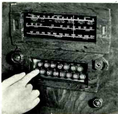
Fig. 4. The word "Automatic" will become illuminated if any button is depressed.
