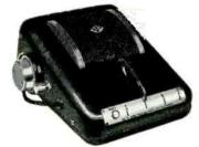
Call-Phone which is equipped with an earphone. Raising the earphone from its rest makes conversation confidential by bringing the other party's voice over the ear-phone instead of the loudspeaker. Other units in the system include the Standard Call-Phone, which has no earphone, the Switchboard Call-Phone for use by telephone operator in extensive installations, and the Paging Call-Phone which ampli-fies the call over large areas.
