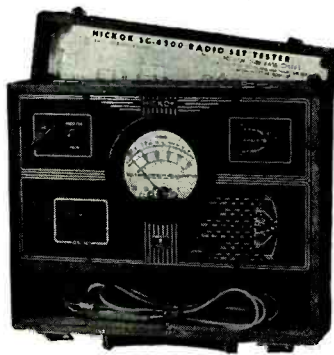
Hickok 4900 set tester, illustrated above, uses the zero-current voltmeter.
