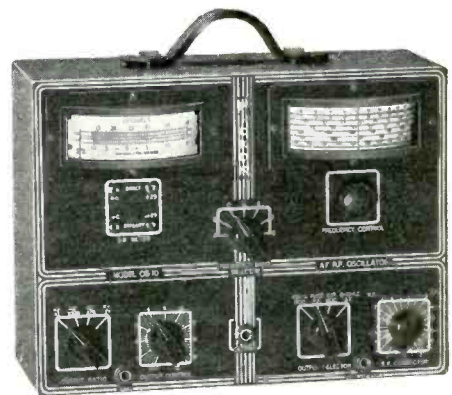
The Hickok OS-10 oscillator used in making the measurements discussed herein.
