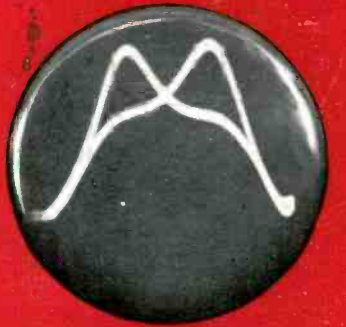
In seeking for the results of No. 3 with a meter, you're apt to do this—peak the transformers at different frequencies
