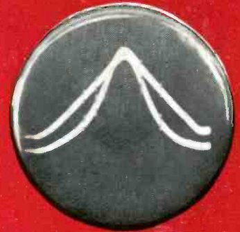
This amplifier was aligned with output meter. Oscillograph shows distortion
