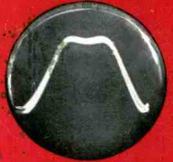
Proper alignment of amplifier that is overcoupled, showing broad peak
