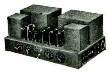
voltage amplifier, two 6F6 triodes as "Power-Drivers" and four 6F6 output tubes. The amplifier will deliver 38 watts a-f normal and 45 watts in continuous heavy-duty speech service. The amplifier includes a two-position input mixer with universal impedance, main gain control, tone control, a-c switch, a-c convenience outlet and dual output of 500 ohms and 15 ohms tapped at 8 and 4. An input coupler is also available for adapting low-impedance microphones such as velocity and dy-
