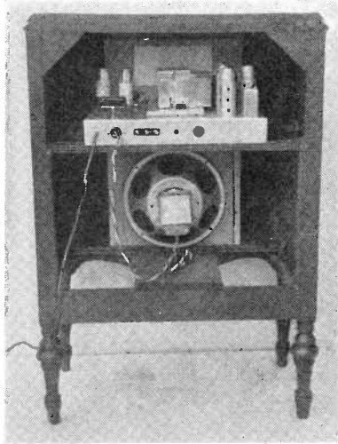
Fig. 3. Behind the scenes with the converted Philco 65. This is one of the simplest receivers to modernize.
