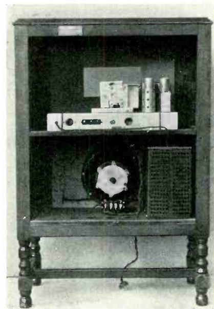
Fig. 4. After modernization. The power pack, as will be observed, has been retained.
