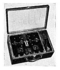
super-sensitive Neon Glow Discharge Tube, which has a two-color scale; this scale indicates at a glance whenever a tube is in good or bad condition. Only four sockets, a 4, a 5, a 6 and a 7-7, are em-ployed in order to simplify the handling of tubes. There are two spares for future tubes and it is also designed to prevent obsolescence.
