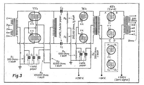
Circuit of the Class A-B amplifier audio channel. Either two or four 45s may be used.
