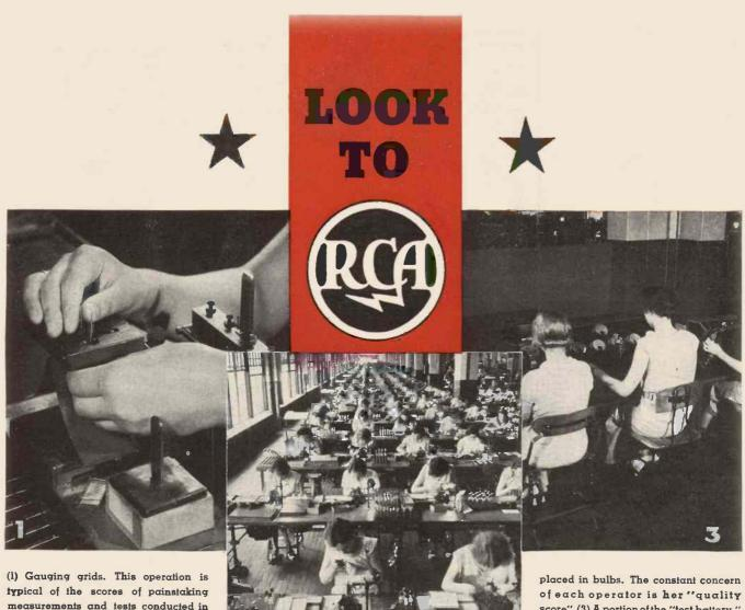
measurements and tests conducted in the Parts Assembly Section. (2) A view of the General Assembly Section. Here the mounts are assembled before being placed in bulbs. The constant concern of each operator is her "quality score".(3) A portion of the "test battery," through which every RCA Cunningham Radiotron must successfully pass before being packed for sale.
