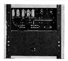
Illustrating the accessibility of all wiring when panel is removed. Removal of panel does not necessitate removal of amplifier or power unit from rack. This photo also shows the spring cradle mounting for the voltage amplifier tubes.
