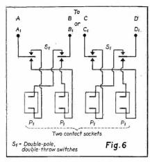
The switching circuit used to change from series to parallel mixer.
