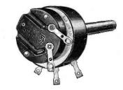
for the resistance element which cannot flex or warp out of line with the contact arm, thus making the mechanical strength of the unit, the electrical stability and wearing qualities exceptional, it is said.
