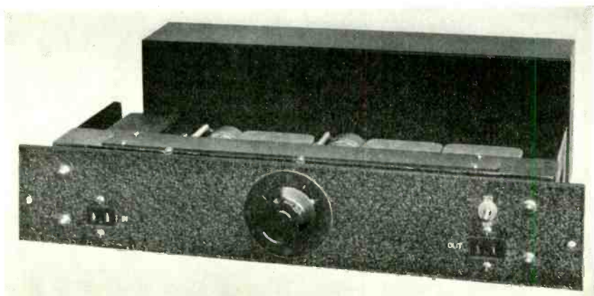
Fig. 5. The pre-amplifier, with dust cover, for rack mounting.
