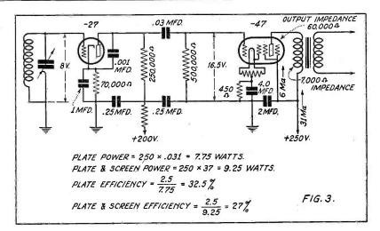
Circuit with pentode power tube which, because of the high amplification factor of the pentode, requires no intermediate audio stage and works direct from the detector
