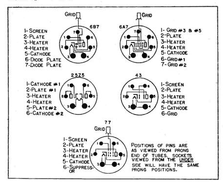
Fig. 6. Prong connections of the tubes used in the Colonial Models 250, 279 and 300 receivers. These connections are standard . . . keep them for reference
