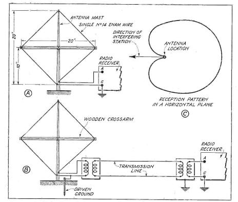
Constructional details and circuit connections of the directional antenna for broadcast reception
