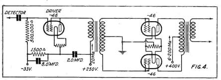
Circuit of a Class B amplifier using one type 46 as a Class A driver and two type 46's in Class B connection, the two latter tubes operating at zero bias
