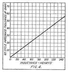
With the inductance of a transformer winding once known, the impedance at 60 cycles can be determined from this curve
