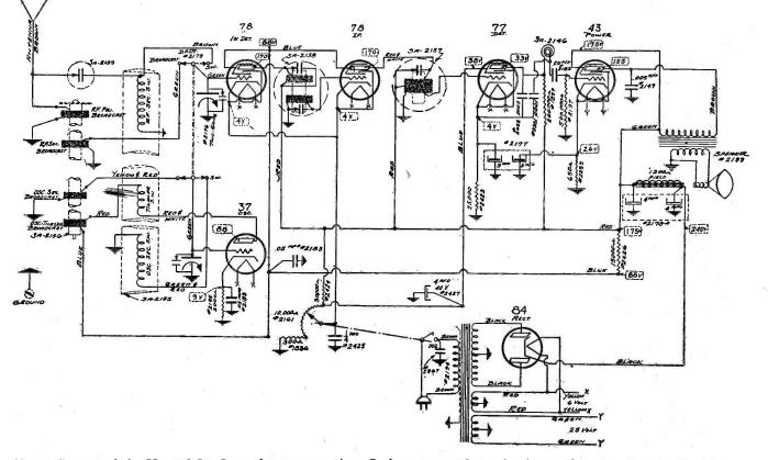
Circuit diagram of the Howard J-3 Super for a-c. operation. Resistance, capacity and voltage values are given on the diagram
