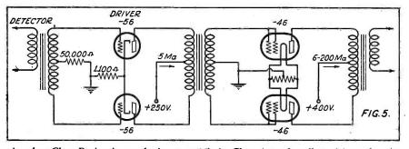
Another Class B circuit, employing two 56's in Class A push-pull as drivers for the 46's. Typical voltage and current values are given
