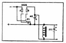
Fig. 3. Circuit of rectifier and filter when receiver is operated from direct current
