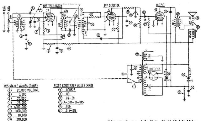
Schematic diagram of the Philco Model 57 A-C. Midget receiver. This job is similar to the former Model 80 except that the new type tubes are employed
