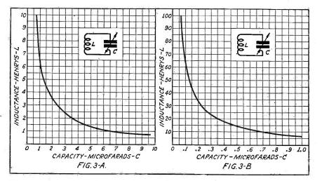
The two curves above give the inductance in henrys of transformer windings corresponding to the various capacity values as used in the circuit of Fig. 2
