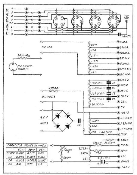
Circuit diagram and values of condensers and resistors for the new Supreme Model 333 Analyzer
