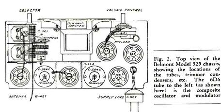
condenser should be at the maximum capacity position—at the extreme right of its rotation.
