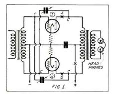
Neutralizing-condenser method of stopping oscillation in the circuits of a pushpull amplifier
