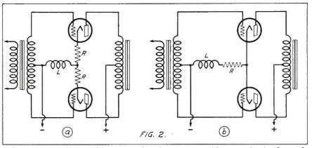
A low-resistance choke coil L connected in the common grid return circuit of a pushpull amplifier is another cure for oscillation. Two methods are shown
