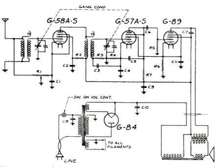
Here is the circuit of the new Majestic Model 380 Midget receiver. This is for a-c. only, with heaters connected in parallel
