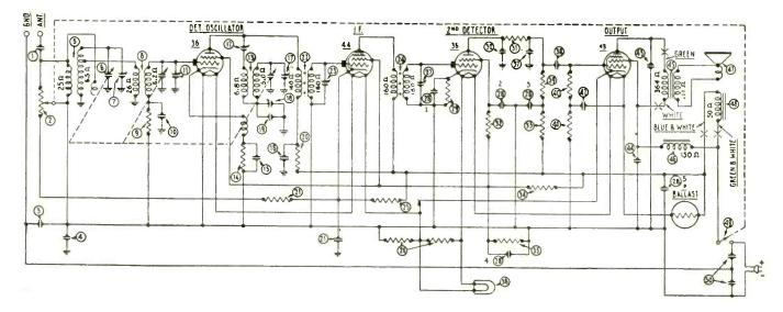
Circuit diagram of the Philco Model 48 D-C. receiver using series heater connection which includes the field of the dynamic speaker
