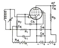
Fig. 3. The 2B7 or 6B7 used as a halfwave rectifier and audio amplifier. The two diode plates are connected together Cathode current cutoff at grid bias volt-
