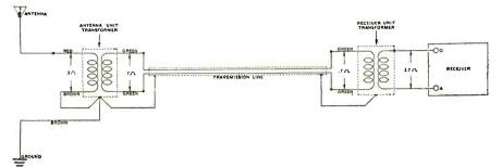
Here is the connection diagram of the Atwater-Kent Type 2-E Interference Eliminator for use in connection with broadcast receivers. The resistance values are given
