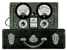
The Ohmmeter is not battery-operated, but is operated in conjunction with a vacuum tube rectifier contained in the case. No rectifier is used with the a-c. voltmeter. This voltmeter works directly from the a-c. line in connection with a voltage adjuster for precise calibration which is independent of line fluctuation.
