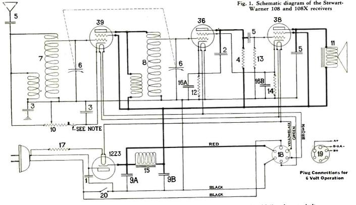
NOTE: In some receivers, a 140 ohm, ½ watt carbon resistor, part 81646 is connected in series with the volume control; in other sets this resistor is built into the volume control.
