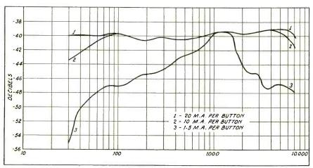
Three curves showing the effects on frequency response of a double-button carbon microphone with changes in button current
