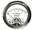
used, it is said. The aluminum needle and other parts are ribbed and made unusually strong throughout. The moving coil is light in weight. The scales are extra long, uniform and easy to read. Sealed cases of one-piece construction means strength and absence of foreign materials.
