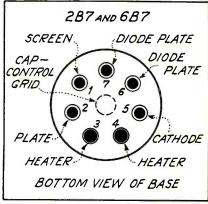
Fig. 5. Base connections for the 2B7 and 6B7 tubes. This is the new small sevenpin base
