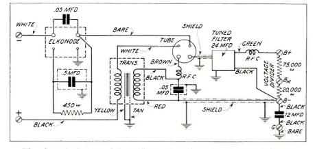
The schematic diagram of the Mallory auto B-Eliminator, using the Elkonode
