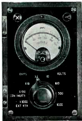
Panel view of the Shallcross Quick-Change Volt-Ohmmeter, all functions of which are controlled by a single rotary switch
