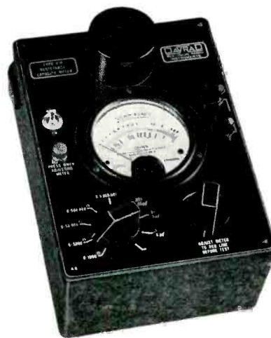
Panel view of the Dayrad Type 870 Test Meter. The dome cap at the rear of the panel covers the rectifier tube
