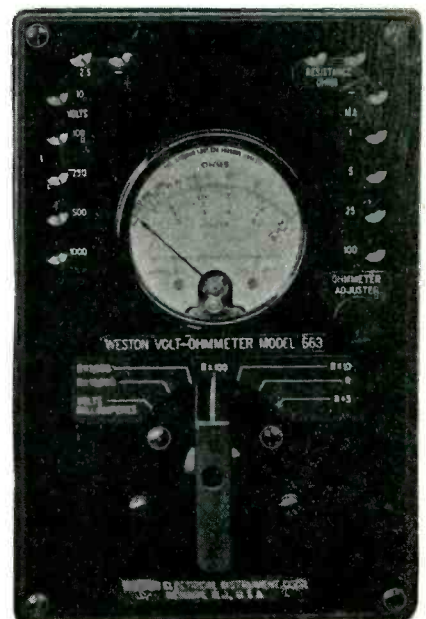
Front panel view of the Weston Model 663 Volt-Ohmmeter. The meter has scales for reading ohms, volts and milliamperes in various ranges
