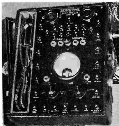
Fig. 4. The Supreme Model 56 Analyzer. One meter is used for all measurements
