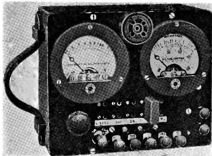
Fig. 7. The Hickok Ohm Capacity Voltmeter which operates direct from a-c. line
