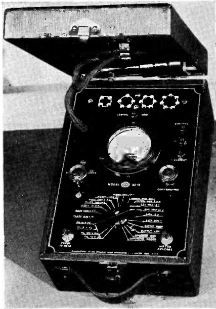
Fig. 17. The Franklin 33-B Set Analyzer, with single meter for all a-c. and d-c. readings
