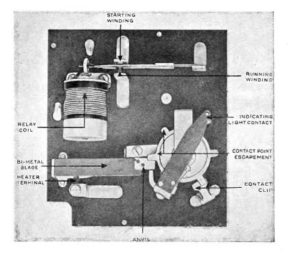
Overload Trip and Starting Relay Devices Model 100 Unit Part No. 20600
