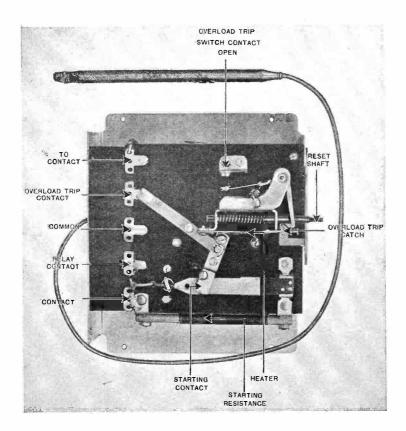
Overload Trip Assembly Models 101 and 103 Part No. 21975
