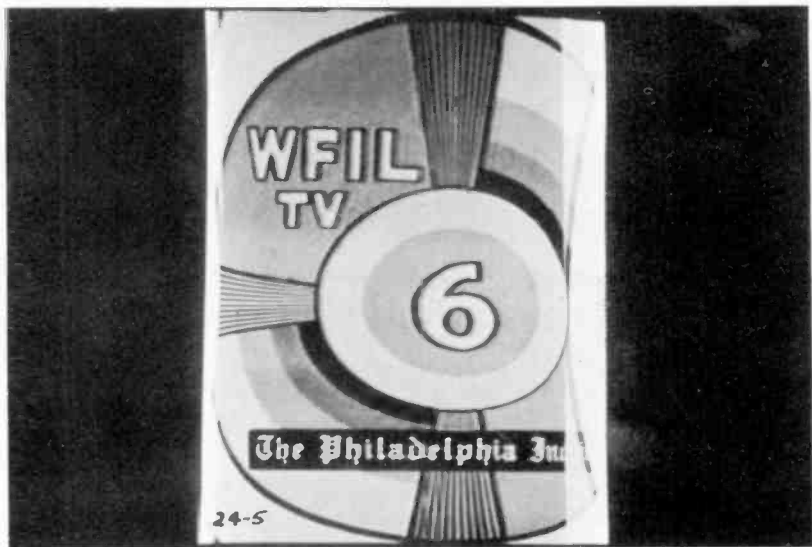
Fold-over at left and right sides of raster produced by leakage of 400,000 ohms across grid coupling capacitor in circuit shown on HD-14.
