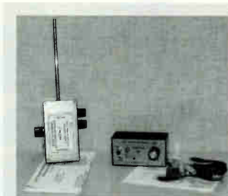
As profiled in the January 1997 issue of Monitoring Times , two popular VLF units are the S.P. McGreevy handheld (left) and the Low Frequency Engineering Unit with tree-tapping probes and a belt loop.
