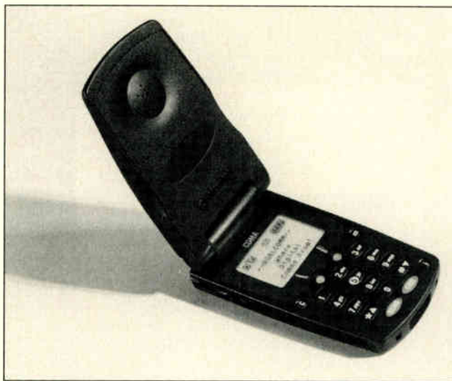
Qualcomm's "Q" phone (above) is the world's smallest and lightest CDMA digital PCS 1900 MHz phone, weighing about 5 ounces. At right is the Qualcomm 1900 MHz CDMA digital PCS/800 MHz analog phone.
