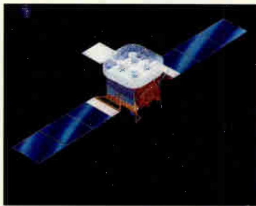
A version of the HS 601 body stabilized satellite.
