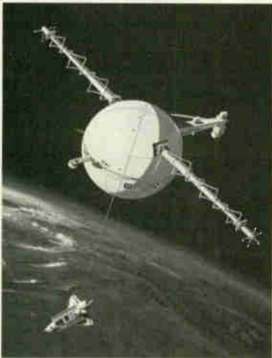
Artist rendition of the Tethered Satellite System deployed from the space shuttle. (Photo courtesy of NASA)
