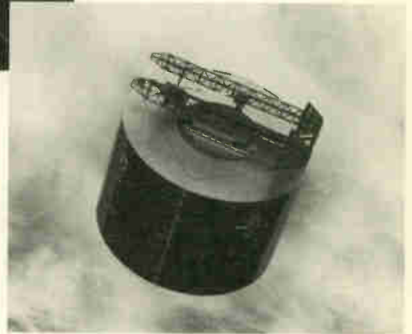
DoD's first two MACSATs (above) were stacked and launched together on a Scout launch vehicle. They were placed into a circular, polar orbit at 720 km. (Photo courtesy of the Department of Defense). At right, Leasat, also known as Syncom, are leased military satellites that use the 240 to 270 Mhz band for military tactical communications. (Photo courtesy of NASA)
