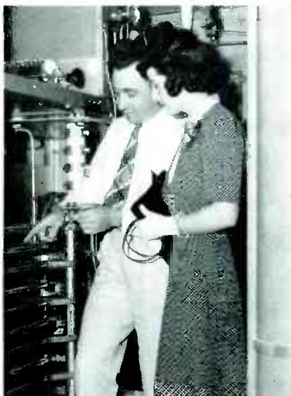
"If a moth flies between these condenser plates," WCKY's Chief Engineer Topmiller tells Miss Virginia Frederick, "both the station and the moth are put out of commission." Mr. Topmiller is comparing the size of a receiving set condenser, which he holds in his hand, with the size of the gigantic transmitter condenser to which he points.
