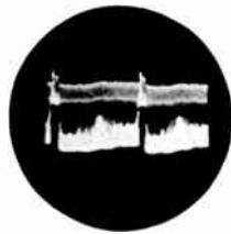
← FIG. 3 Cathode of video detector (pin 1 of V-9-A, 6AL5) 50 volts peak-to-peak—60 cps.
