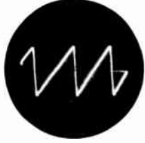
← FIG. 11 Plate of horizontal sweep oscillator (pin 2 of V-2, 6SN7-GT) 80 volts peak-to-peak—15,750 cps.
