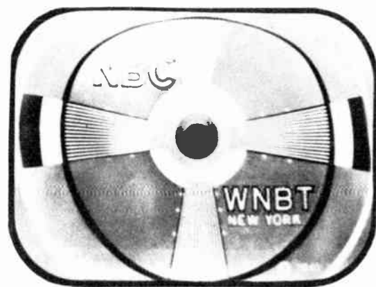
FIG. 9: VERTICAL LINEARITY MISADJUSTED
