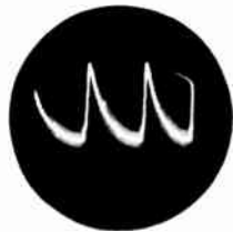
← FIG. 9 Plate and cathode of horizontal phase detector (pin 1 or 2 of V-6, 6AL5) 13 volts peak-to-peak—15,750 cps.
