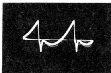
Figure 64—Input of Vertical Deflection Coils (75 Volts PP) (Junction of Green Lead of T108 and Green Lead of Yoke)
