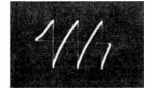
Figure 35—Horizontal Oscillator Output (60 Volts, P to P) (Junction of C75 and C77)
