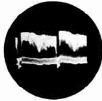
← FIG. 4 Grid of Kinescope (pin 2 of V-5) 40 volts peak-to-peak—60 cps.
