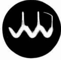
← FIG. 10 Grid of horizontal sweep oscillator (pin 1 of V-2, 6SN7-GT) 43 volts peak-to-peak—15,750 cps.
