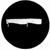
← FIG. 5 Plate of sync clipper (pin 1 of V-7-B, 12AU7) 12 volts peak-to-peak—60 cps.
