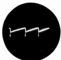
← FIG. 15 Plate of vertical sweep oscillator output (pin 1 and 6 of V-1, 12AU7) 600 volts peak-to-peak—60 cps.
