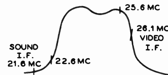
FIG. 4- OVER-ALL I-F RESPONSE CURVE.
