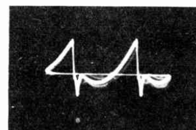
Figure 59—Input of Vertical Deflection Coils (75 Volts PP) (Junction of Green Lead of T108 and Green Lead of Yoke)
