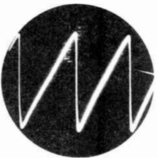
ACROSS C172, .0018 MFD, HORIZ. OSCILLATOR OUTPUT 'SCOPE AT 5250 C.P.S. 75V. P-P
