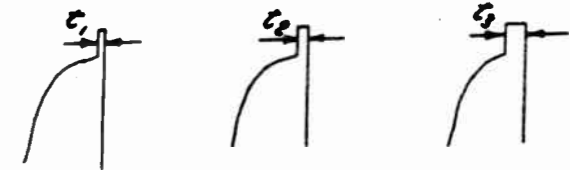
FIGURE 8 - VARIATION IN SYNC PULSE DURATION
