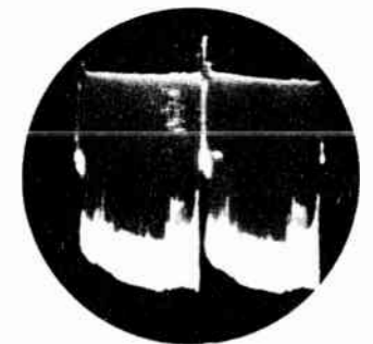
CONTROL GRID, PICTURE TUBE 'SCOPE AT 30 C.P.S. 60V. P-P. VARIATION WITH PICTURE CONTROL.
