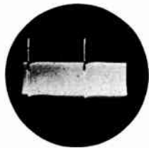
← FIG. 6 Plate of sync amplifier (pin 6 of V-22-B, 12AU7) 20 volts peak-to-peak—60 cps.
