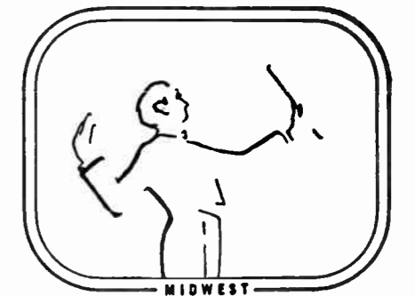
Loss of detail - caused by excessive signal
