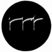
← FIG. 13 Grid of vertical sweep oscillator (pin 2 of V-22-A, 12AU7) 150 volts peak-to-peak—60 cps.
