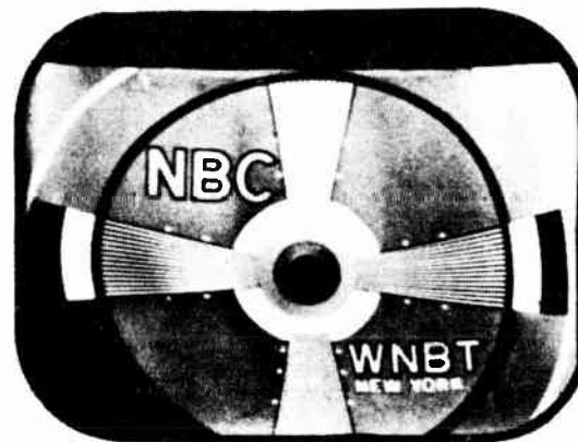
FIG. 5: FOCUS COIL AND ION TRAP MISADJUSTED
