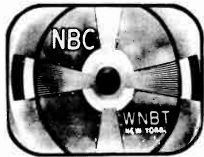
FIG. 5. HEIGHT CONTROL MISADJUSTMENT
