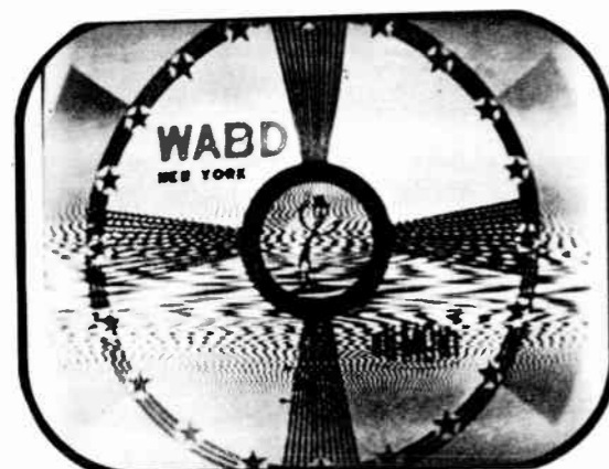
FIG. 37: DIATHERMY INTERFERENCE - MEDIUM
