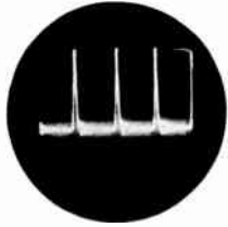
← FIG. 12 Plate of AGC (pin 5 of V-24, 6AU6) 160 volts peak-to-peak—15,750 cps.
