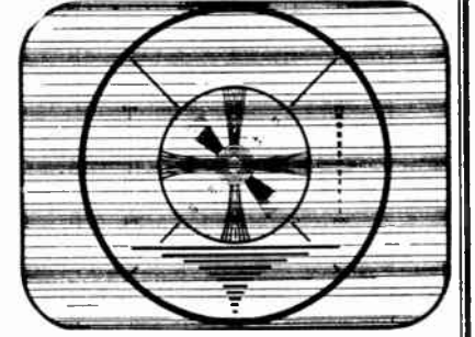
FIG. 3 — SOUND INTERFERENCE CAUSED BY INCORRECT TUNING
