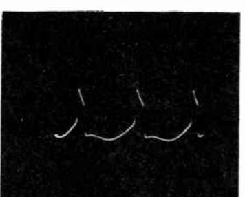
Figure 25. Vertical-Output Plate, Plate Cap 450 volts, 60 c.p.s.
