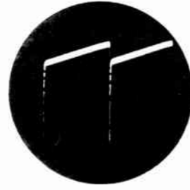
(Yellow lead) deflection yoke, 120 V. p/p, 'scope at 30 c.p.s.
