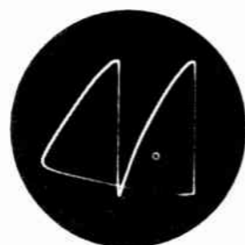
Grid of 6BQ6, 55 V. p/p, 'scope at 7875 c.p.s.
