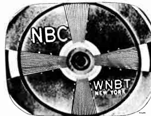
Figure 19—Horizontal Linearity Control Misadjusted (Picture Cramped in Middle)
