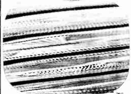
Figure 26—Test Pattern Showing Out of Sync Condition When Horizontal Hold Control Is in a Counter-clockwise Position—Just Before Pulling Into Sync
