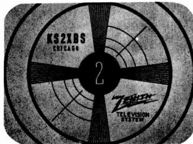
Fig. 9 Receiver Correctly Adjusted On Test Pattern.
