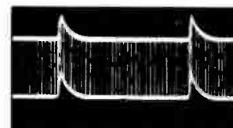
12AX7 (V14) Hor. Sync Separator and AGC Rectifier Plate (Pin 1) 45 Volts (PP) Vertical
