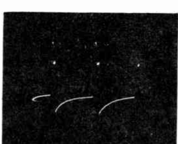
Figure 27. Phase-Splitter Cathode, Pin 8 9 volts, 15,750 c.p.s.
