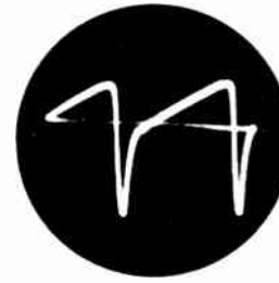
Grid of Hor. Output (junction of R-202, R-203), 'scope at 7875 c.p.s. 150 V. p/p.
