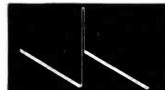
6AH4GT (V17) Vertical Output Plate (Pin 5) 700 Volts (PP) Vertical
