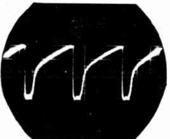
13. (V-17) Horizontal Output, Grid, (Pin 1) 15750 C.P.S., 200 V.P.P.
