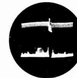
Grid of 1st Sync Ampl., pin 1, V-112A, 'scope at 30 c.p.s. 18 V. p/p.
