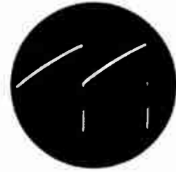
Grid of Vert. Output, pin 5, V-114, 'scope at 30 c.p.s. 50 V. p/p.
