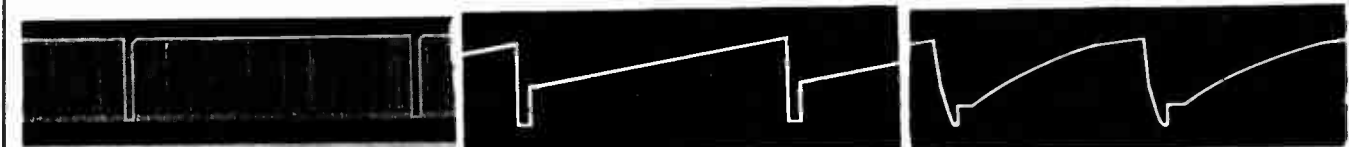
No. 8—6SN7 Vert. Output Grid 120V P-P 60 C.P.S.
