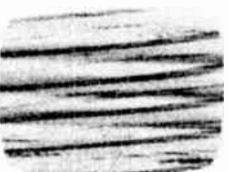
Misadjusted Horizontal Hold
