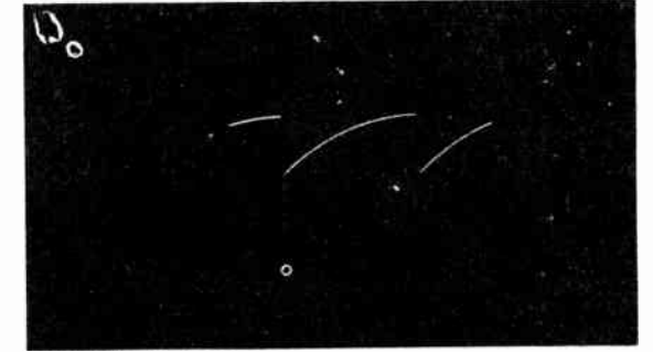
Figure 19. Vertical-Output Grid, Pin 2 120 volts, 60 c.p.s.
