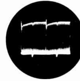
Cathode of Sync Clipper, pin 3, V-113A, 'scope at 30 c.p.s. vert. osc. unsynchronized. 50 V. p/p.
