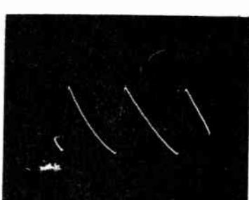
Figure 22. Vertical-Oscillator Grid, Pin 2 170 volts, 60 c.p.s.
