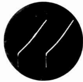
Grid of vertical output, 18 V. p/p, 'scope at 30 c.p.s.
