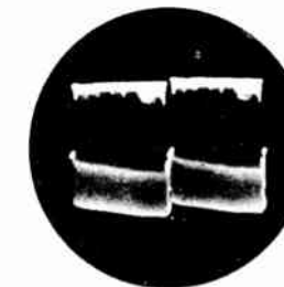
Control grid of picture tube, 'scope at 30 c.p.s. 50 V. p/p.**
