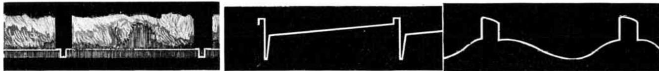
No. 3—Pix Tube Grid 20-100V P-P 60 C.P.S.
