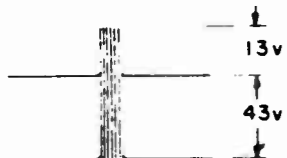
OUTPUT OF 2 nd SYNC AMPLIFIER AT PIN 2 OF V117 (6SN7) (60~)
