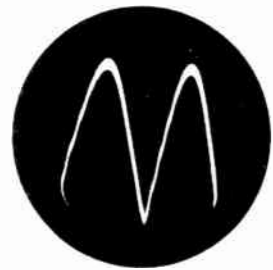
Cathode of damper, 50 V. p/p, 'scope at 7875 c.p.s.
