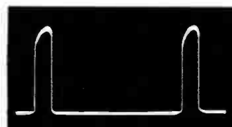
12AU7 (V15) Sync Amplifier and Clipper Plate (Pin 1) 80 Volts (PP) Horizontal
