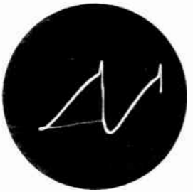
Junction of C405 & R409 through capacitor, 25 V. p/p, 'scope at 7875 c.p.s.
