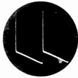
Plate of vertical output, 750 V. p/p, 'scope at 30 c.p.s.
