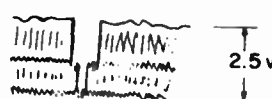
VIDEO SIGNAL OUTPUT OF PIX 2 nd DETECTOR AT JUNCTION OF L188 AND R139 (60~)
