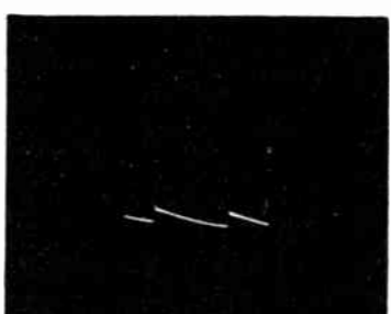
Figure 25. Vertical-Output Plate, Plate Cap 450 volts, 60 c.p.s.
