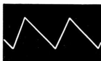
6AL5 (V15) Horizontal Phase Detector (Pin 1 or 2) 9 Volts (PP) Horizontal
