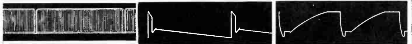
No. 6—12AT7 Phase Splitter Cathode 18V P-P 60 C.P.S.
