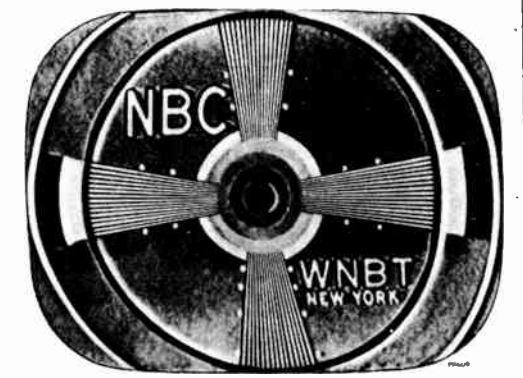
Figure 21—Horizontal Drive Control Misadjusted
