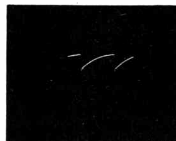
Figure 24. Vertical-Output Grid, Pin 5 40 volts, 60 c.p.s.
