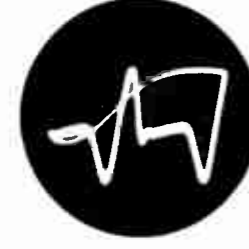
Plate of Hor. Osc., pin 1, V-117A, 'scope at 7875 c.p.s. 28 V. p/p.
