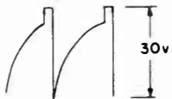
SINE WAVE PLUS HORIZONTAL SYNC PULSE AT TERMINAL F OF T108 SYNC DISCRIMINATOR TRANSFORMER (15,750~)
