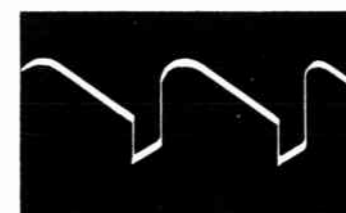
6AL5 (V15) Horizontal Phase Detector (Pin 7) 28 Volts (PP) Horizontal
