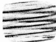
Misadjusted Horizontal Hold
