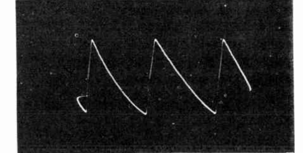
Figure 28. Phase Comparator, Pins 5 and 7 6 volts, 15,750 c.p.s.
