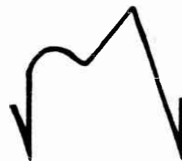
STABILIZING COIL FREQUENCY TOO HIGH
