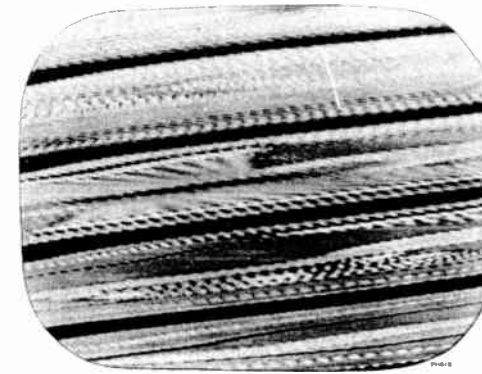
Figure 23—Test Pattern Showing Out of Sync Condition When Horizontal Hold Control Is in a Counter-clockwise Position—Just Before Pulling Into Sync
