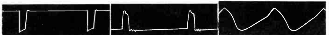
No. 6—12AT7 Phase Splitter Cathode 18V P-P 15,750 C.P.S.
