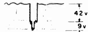
VIDEO SIGNAL OUTPUT TO GRID OF KINESCOPE AT JUNCTION OF L192 AND C151 (60~)
