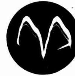
Cathode of Damper, pin 3, V-120, 'scope at 7875 c.p.s. 40 V. p/p.
