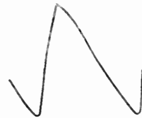
6AL5 HORIZ. PHASE DET. PIN 1 & 2 15,750 CYCLES 11 VOLTS PP
