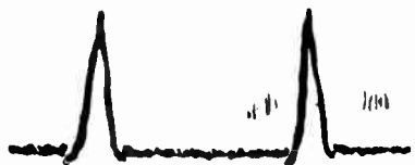
PIN 6 (V9B) 12AU7 SYNC. CLIPPER (HORIZ. SCOPE) 65 VOLTS PP
