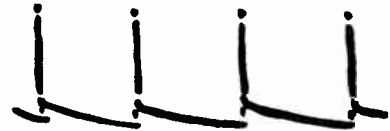
PIN 9 (V15) 6S4 VERTICAL OUTPUT 850 VOLTS PP
