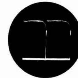
Grid of sync clipper, 25 V. p/p, 'scope at 30 c.p.s.
