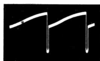
6AH4GT (V14) Vertical Output Grid (Pin 1) 80 Volts (PP) Vertical
