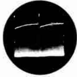
Plate of 2nd Sync Ampl., pin 5, V-112B, 'scope at 30 c.p.s. 115 V. p/p.
