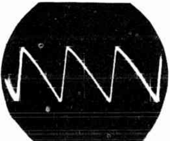
10. (V-14) Phase Detector, Cathode, (Pin 1) 15750 C.P.S., 7 V.P.P.
