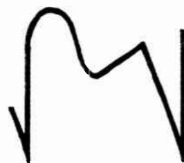
STABILIZING COIL FREQUENCY TOO LOW
