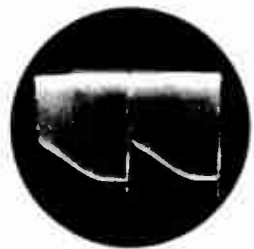
Plate of 1st Sync Ampl., pin 2, V-112A, 'scope at 30 c.p.s. 18 V. p/p.
