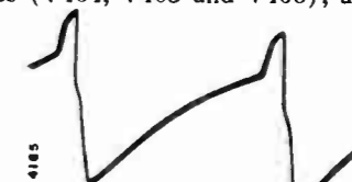
Figure 11. Waveform on Grid Pin 1 of V403 With Sync Pulse.
