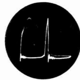
A.G.C. plate, 450 V. p/p, 'scope at 7875 c.p.s.
