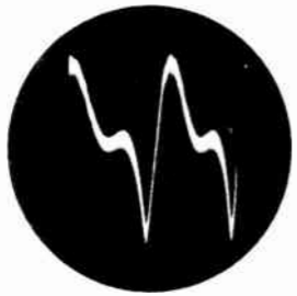
Output of horizontal linearity, 40 V. p/p, 'scope at 7875 c.p.s.
