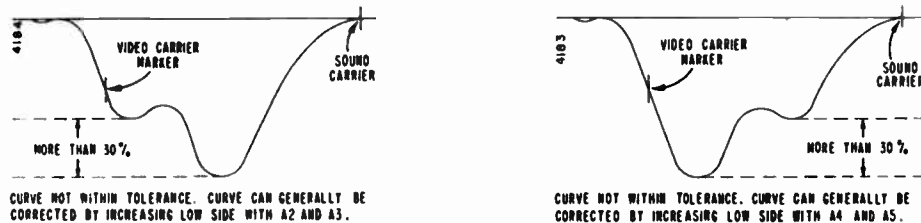
Figure 27. Over-all RF and IF Response Curves, Incorrect Shape.
