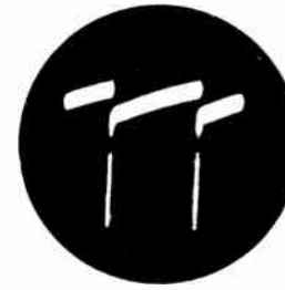
Secondary of Vert. Output trans., yellow lead, 'scope at 30 c.p.s. 105 V. p/p.
