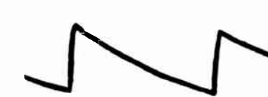
PIN 5 & 7 (V10) 6AL5 HORIZ. PHASE DETECTOR 16 VOLTS PP
