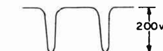
OUTPUT OF PLATE CIRCUIT OF HORIZONTAL OSCILLATOR AT PIN 3 OF V121 6K6 (15,750~)
