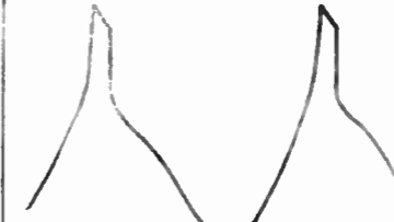
6SN7GT HORIZ. OSC PIN 1 15,750 CYCLES 40 VOLTS PP
