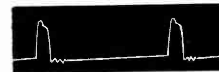
No. 10—Term "A" Hor. Output Transformer 450V P-P 15,750 C.P.S.
