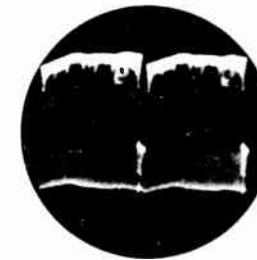
Grid of 1st Video Ampl., pin 1, V-110A, 'scope at 30 c.p.s. 5 V. p/p.*
