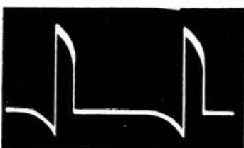
Junction of R207 and R209 27 Volts (PP) Horizontal
