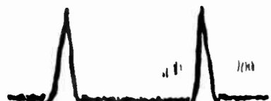
PIN 6 (V9B) 12AU7 SYNC. CLIPPER (HORIZ. SCOPE) 65 VOLTS PP
