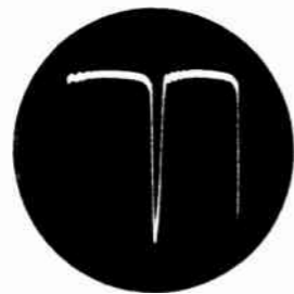
Pin 5 (horizontal) output, 140 V. p/p, 'scope at 7875 c.p.s.
