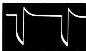
12AU7 (V12) Sync Amplifier Cathode (Pin 3) 27 Volts (PP) Horizontal
