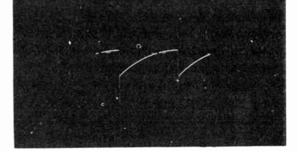
Figure 24. Vertical-Output Grid, Pins 2 and 7 120 volts, 60 c.p.s.
