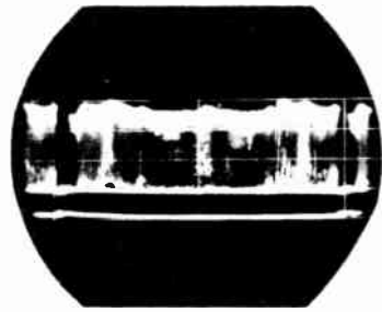
1. (V-11) 1st Video, Grid, (Pin 1), 60 C.P.S., 2.5 V.P.P.
