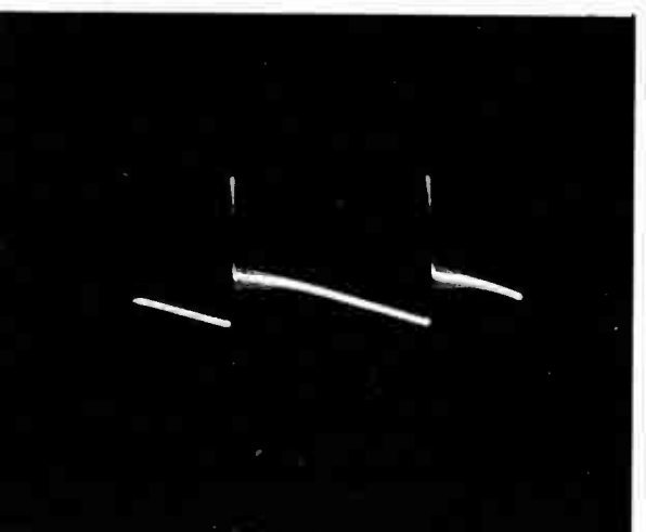
Figure 23. Vertical-Output Plate,* Pin 9 450 volts, 60 c.p.s.
