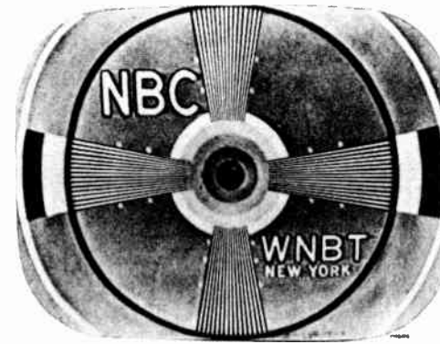
Figure 18—Focus Magnet and Ion Trap Magnet Misadjusted
