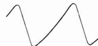
Figure 12. Waveform on Grid Pin 1 of V403 Without Sync Pulse.
