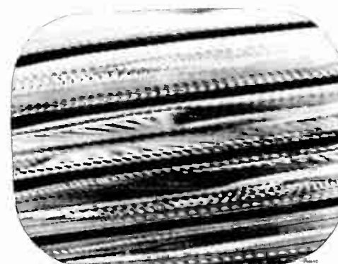
Figure 23—Test Pattern Showing Out of Sync Condition When Horizontal Hold Control Is in a Counter-clockwise Position—Just Before Pulling Into Sync
