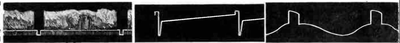
No. 3—Pix Tube Grid 20-100V P-P 60 C.P.S.
