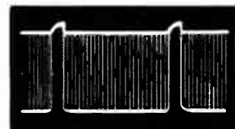
12AU7 (V15) Sync Amplifier and Clipper Plate (Pin 1) 90 Volts (PP) Vertical
