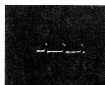
Figure 15. Gated-Level Grid, Pin 2 3 volts, 15,750 c.p.s.
