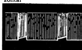
12AU7 (V12) Sync Separator Plate (Pin 6) 60 Volts (PP) Vertical
