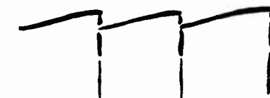
PIN 6 (V15) 6S4 VERTICAL OUTPUT 48 VOLTS PP
