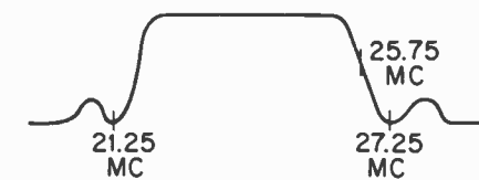
(A) TYPICAL NORMAL VIDEO I-F RESPONSE CURVE
