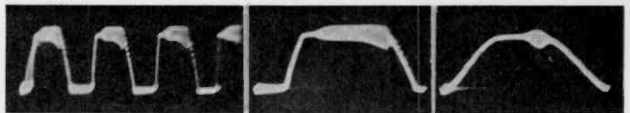
Figs. 1, 2 and 3. Fig. 1 (left) shows a transient oscillation in a Class B amplifier. Note that the oscillation is more clearly evident with a single cycle on the screen, see Fig. 2. Fig. 3 (right) shows a single cycle of the output voltage for decreased grid excitation
