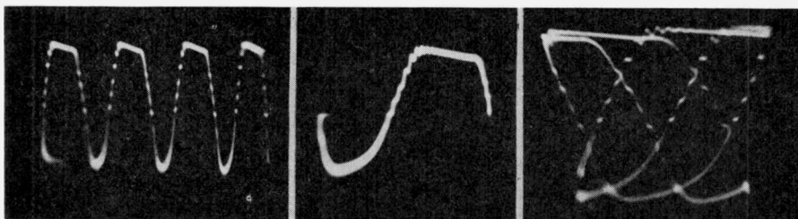
Figs. 9, 10 and 11. An audio wave with a superimposed transient, as indicated by the "dots," is shown in Fig. 9 (left). One cycle of the wave is shown in Fig. 10. Note how the detail of the transient is brought out in Fig. 11 by the use of a higher sweep frequency
