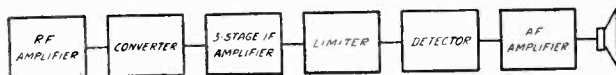
FIG. 1.—Block diagram of a receiver designed for the reception of frequency-modulated signals. With the exception of the limiter stage, the lineup is similar to that of a conventional superheterodyne receiver.
