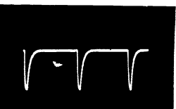
④ TP-5 SYNC PLATE HORIZONTAL RATE 60V P-P
