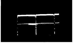
16 V105 PIN 3 KINESCOPE 1ST ANODE VERTICAL RATE 130V P-P
