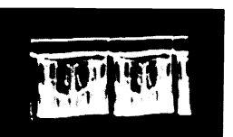
⑦ V205B PIN 9 VIDEO AMPLIFIER PLATE VERTICAL RATE 110V P-P
