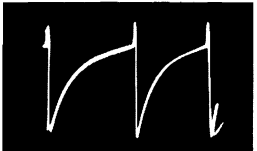
⑤ V206B PIN 9 VERTICAL OSCILLATOR GRID VERTICAL RATE 180V P-P
