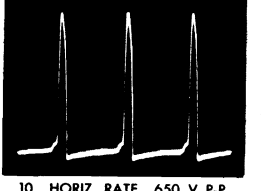
10 HORIZ. RATE 650 V P-P TERM. A PW500 AGC PLATE
