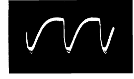
18 SR201 ANODE HORIZONTAL PHASE DETECTOR HORIZONTAL RATE 15V P-P
