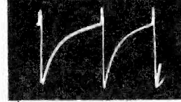
5 VERT. RATE 180V P-P V206B PIN 9 VERTICAL OSCILLATOR GRID
