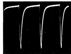
7 HORIZ RATE 65 V P-P V501B PIN 1 SYNC AMPLIFIER PLATE
