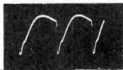
11 VERT. RATE 12V P-P SR201 CATHODE JUNCTION HORIZONTAL PHASE DETECTOR
