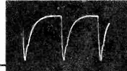
2 HORIZ. RATE 130V P-P V101 PINS 2 & 6 HORIZONTAL OUTPUT GRID
