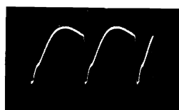
HORIZ. RATE 12V P-P SR201 CATHODE JUNCTION HORIZONTAL PHASE DETECTOR
