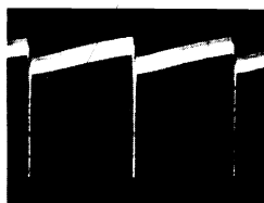
15 VERT. RATE 110 V P-P PIN 1 J101 (YOKE SOCKET) VERT. OUTPUT TRANS. SEC.
