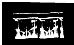
VERT. RATE 90V P-P V205B PIN 9 VIDEO AMPLIFIER PLATE
