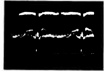
Composite video, 2nd detector output, L8T (on V.O.S. panel), 4.0 volts in "Normal," 7.0 volts in "Fringe," 60 c.p.s.
