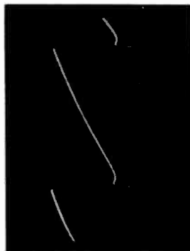
Input of vertical integration network, contact 1 of N1W, 38 volts, 60 c.p.s.
