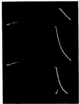
High voltage pulse, loosely coupled to yoke lead, 15,750 c.p.s.
