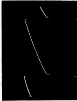
Vertical oscillator plate, pin 6 of 6CS7, 85 volts, 80 c.p.s.
