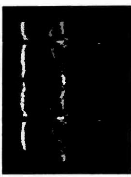
Composite signal, 2nd det. output (L1U of IF panel) or video input (L13Y of video panel), 5 volts, maximum contrast, 60 c.p.s.
