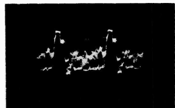
W4 Composite video signal, plate of video amplifier (pin 7, V-6). 110 volts PP. (Oscilloscope synced near horizontal rate)
