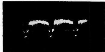
W2 Composite video signal, grid of video amplifier (pin 2, V-6). 4 volts PP. (Oscilloscope synced near horizontal rate)
