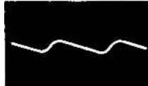
12AX7 (V14) Hor. Sync Separator and AGC Rectifier Cathode (Pin 3) 4.0 Volts (PP) Horizontal
