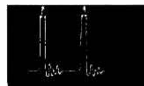
AGC Winding of Horizontal Output Transformer (Point X to Ground) 300 Volts (PP) Horizontal
