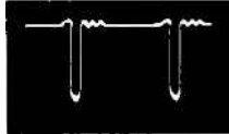
12AX7 (V14) Hor. Sync Separator and AGC Rectifier Plate (Pin 1) 45 Volts (PP) Horizontal
