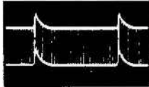
12AX7 (V14) Hor. Sync Separator and AGC Rectifier Plate (Pin 1) 45 Volts (PP) Vertical
