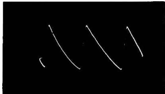
Phase Comparer, Pins 5 and 7 8 volts, 15,750 c.p.s.
