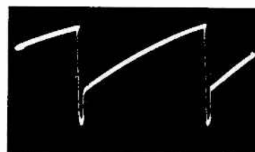
6BL7GT (V14) Vertical Output Control Grid (Pin 4) 95 Volts PP Vertical
