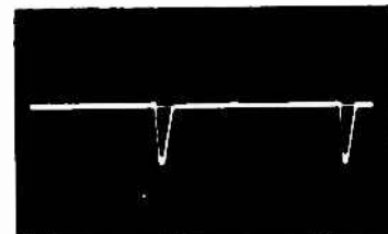
12AX7 (V13) Hor. Sync. Sep. Plate (Pin 6) 37 Volts PP Horizontal
