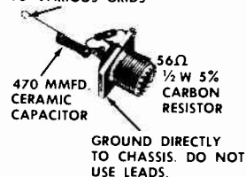
Fig. 6 IF Alignment Fixture
