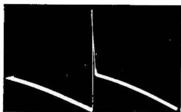
6BL7GT (V14) Vertical Output Plate (Pin 5) 830 Volts PP Vertical
