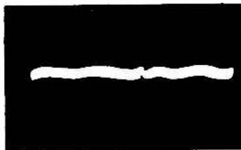
12AX7 (V13) Hor. Sync. Sep. and AGC Rectifier Cathode (Pin 8) 2.6 Volts PP Vertical
