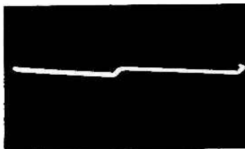
12AX7 (V13) Hor. Sync. Sep. and AGC Rectifier Cathode (Pin 8) 2.6 Volts PP Horizontal
